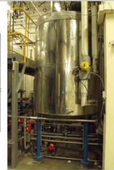
REF CB5268 2X 4,000L, 24BRL, S/S VERTICAL, JACKETED, INSULATED & AGITATED YEAST VESSELS
