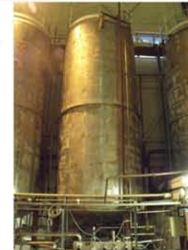
REF CB5245 4X 41,000L, 250BRL, BRIGHT BEER STAINLESS STEEL VESSELS, WP 1.2Bar TP 1.4Bar
