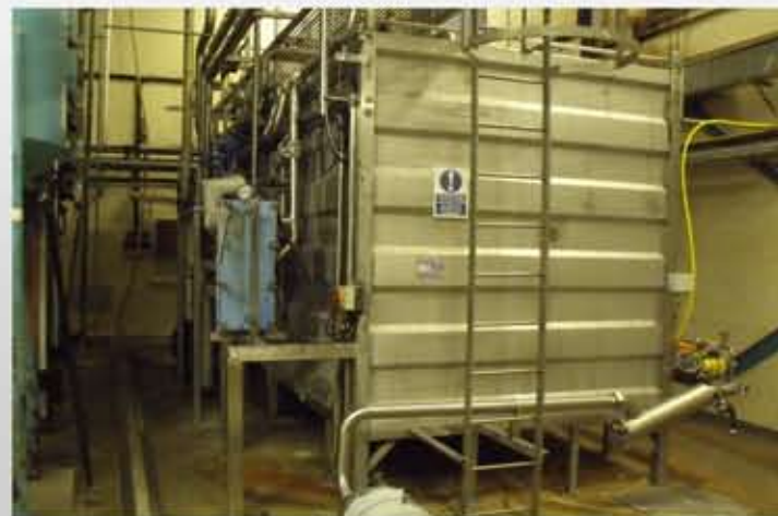
REF M0235 CIP SET WITH 3X RECTANGULAR STAINLESS STEEL TANKS AND APV W+55/35 PUMP
