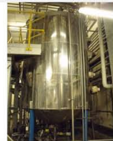
REF CB5272 KALIBER ENG. 8000L, 48BRL, YEAST TANK S/S 316 INSULATED, TWIN JACKETED & AGITATED
