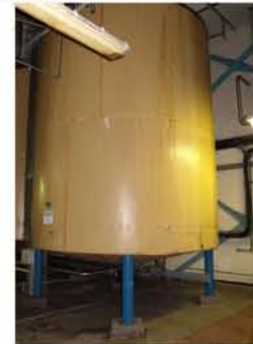
REF CB5260 4X 32,000L, 195BRL, VERTICAL, STAINLESS STEEL, INSULATED VESSELS
