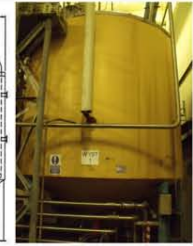
REF CB5273 2X 20,500L, 125BRL, VERTICAL, STAINLESS STEEL, JACKETED, INSULATED & AGITATED VESSELS
