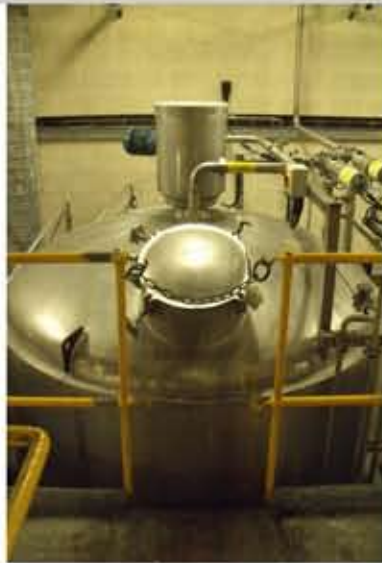
REF CB5264 - 4X 9,000L, 55 BRL, VERTICAL S/S JACKETED & INSULATED AGITATED YEAST VESSELS
