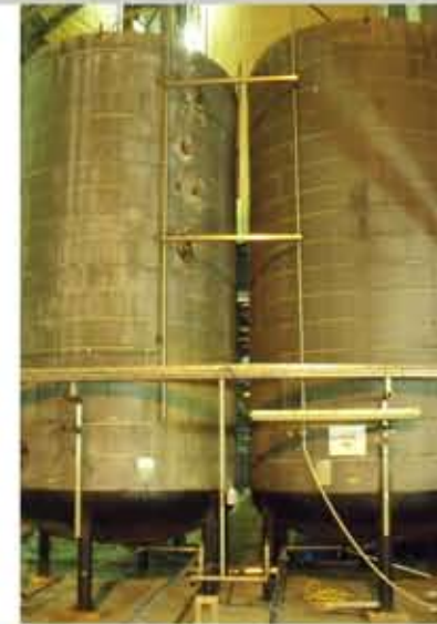
REF CB5249 2X 36,000L, 220BRL, BRIGHT BEER TANKS, S/S, INSULATED & SIDE MOUNTED AGITATOR
