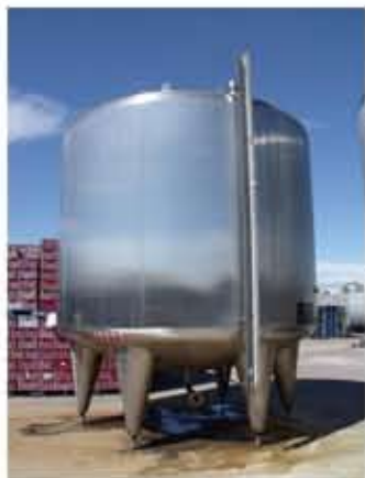
2X 230 BRL, 37,800L STAINLESS STEEL, INSULATED, BRIGHT BEER TANKS
