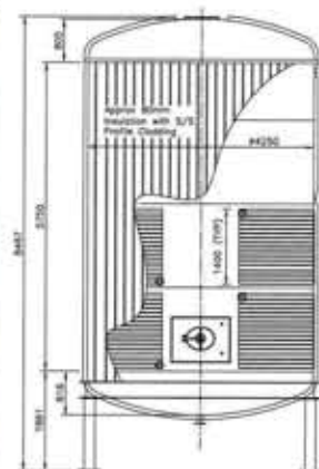
3X BRIGGS 520BRL (WORKING), 95,600L S/S JACKETED, INSULATED, BRIGHT BEER TANKS
