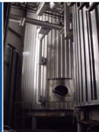
3X BRIGGS 520BRL (WORKING), 95,600L S/S JACKETED, INSULATED, BRIGHT BEER TANKS
